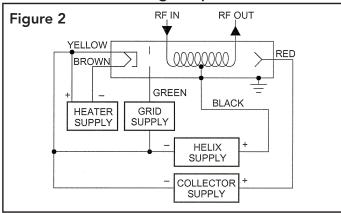
The Ring Loop TWTs are best known for an ability to amplify microwave signals simultaneously over a radar band of frequencies. A Ring Loop TWT is illustrated schematically in Figure 2, which also shows the power supplies to operate the TWT. This TWT consists of an electron gun (composed of a heater, cathode, and control anode), a helix (slow-wave structure), an attenuator, a collector, and an input and an output coupling element
