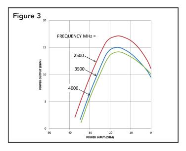
The gain is essentially constant at a given frequency for low RF drive levels, but decreases at higher levels. When the RF electric field becomes too strong, as a result of either amplification or input signal, the amount of energy which the beam can deliver to the wave reaches a maximum limit. This condition, known as the saturation point of the TWT, represents the maximum power which can be delivered for a given condition of beam current. If the input power is increased beyond the value which
