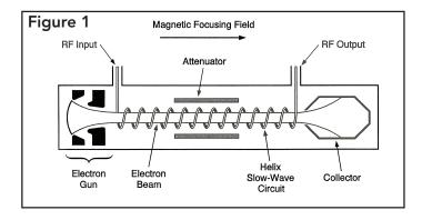
In addition, a magnetic field along the axis of the device (not shown) is used to focus the electron stream. Although TWT's may differ widely in size and construction, depending on the application, the basic theory of operation is the same for all types.
